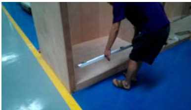
Step 1.Put the double-U channel on the ground.
